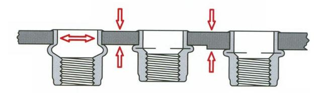
As the internal connector is tightened, the knurled body expands 360° filling hole.
